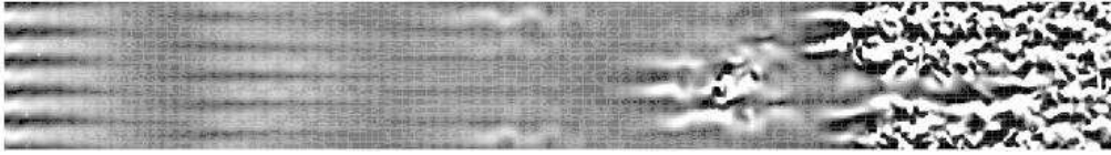
FIGURE 1. Contour plot of streamwise velocity fluctuations in a plane parallel to the wall in the core of the boundary layer during bypass transition induced by free-stream turbulence. The flow is from left to right. DNS simulation by Zaki & Durbin (2004).
