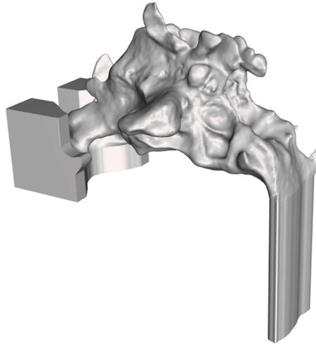
Figure 4: An STL surface mesh file is generated from the segmented CT scan and modified for simulation.
